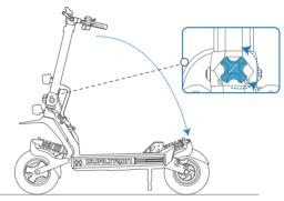
Unscrew the folding knob and M8 screws, then fold the steeing tube. A Risk of pinching!
