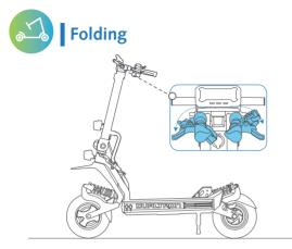
Fold the handlebars,slide the folding handle lock out of position to release handles.
