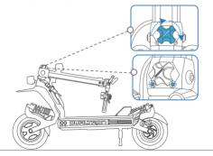
Install back the folding knob prevent loss. Note:Please keep these two M8 screws, they must be installed when unfolding
