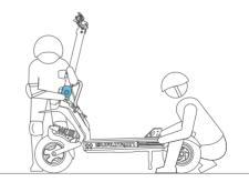
Lift up the bottom of the front fork and rear foot pedestal to carry if necessary. Make sure the scooter is carried by two or more people. Arisk of pinching!
