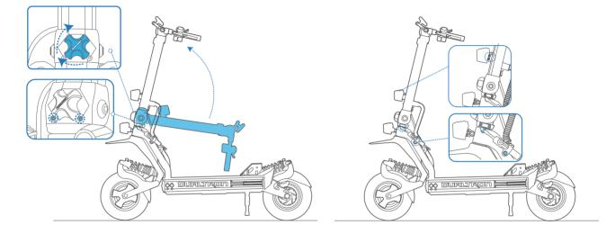
① Unfold the steering tube and lock the folding knob firmly.
