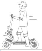
2. Stand on the footboard with one foot and push off with the other foot to start gliding. \*Make sure you have disabled SAFE mode.(SAFE mode setting via Dualtron app.Deactivate safe mode by squeezing brake lever.)
