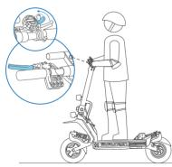
Slow down by releasing the throttle and squeezing brake levers.
