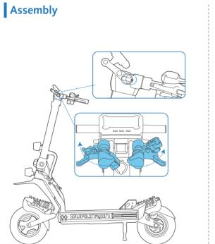
Unfold the handlebars,slide the folding handle lock into position to fix the handle firmly. During use, if the handle is slightly shaken, please unscrew the adjustment screw a little.
