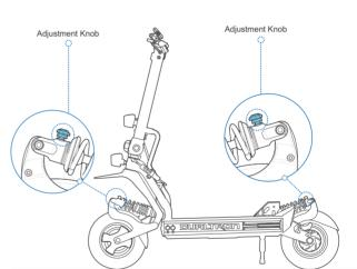
Turn the adjustment knob to the right to increase the shock rebound resistance. Turn the adjustment knob to the left to decrease the shock rebound resistance. Note: The shock is set to the default position before leaving the factory. Please follow the steps above to adjust it according to your riding habits.
